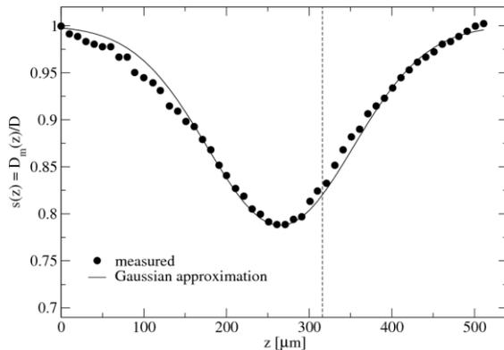
**Figure 3:** Radial scaling function dependence on the distance along the fiber, computed from the measured diameter variation,  $D_m(z)$ , normalized to the nominal fiber diameter,  $D = 125 \mu\text{m}$ .
