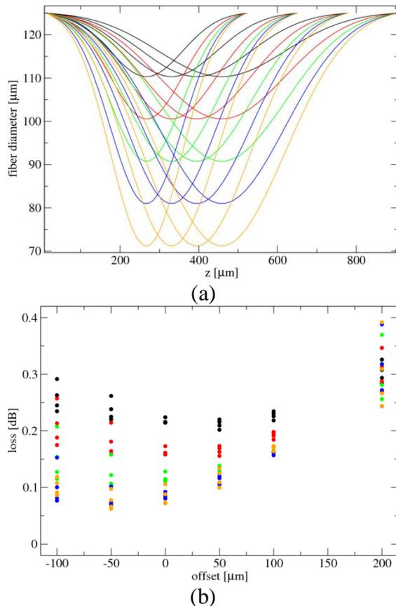
**Figure 5:** (a) Simulated Vascade EX3000 to SMF-28 Ultra taper traces with Gaussian shape and variable depth and width); (b) Corresponding computed splice losses vs. splice point offset from taper minimum.
