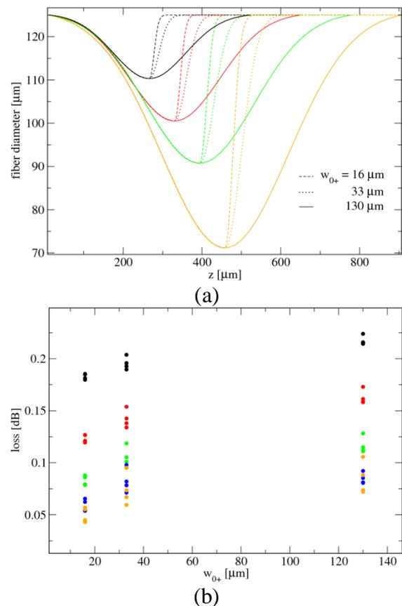
**Figure 6:** (a) Simulated Vascade EX3000 fiber to SMF-28 Ultra fiber taper traces with asymmetric shapes (12 curves are shown as an example); (b) Corresponding splice losses computed for the splice point located at the taper minimum.
