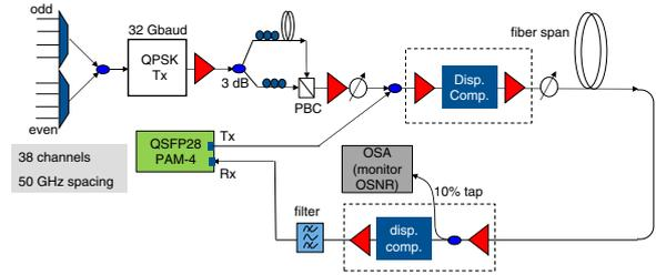
**Fig. 1** Experimental configuration for transmission experiments
