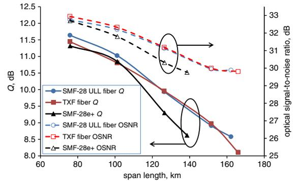
**Fig. 4**  $Q$  and OSNR versus span lengths for each fibre
