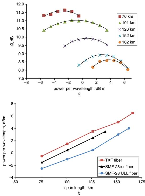
**Fig. 3** PAM-4 transmission data over fibre systems
