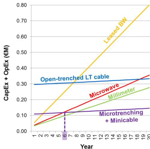
Figure 7. TCO comparison of backhaul solutions using microtrenching and minicable
