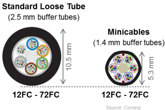
Figure 6. Corning minicables offer 50% reduction of outer cable diameter relative to standard loose tube cable
