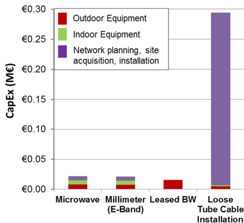
**Figure 2. First installed costs to backhaul a macrocell site using wireless and wireline solutions**
