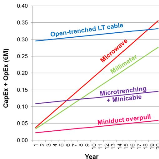
Figure 8. TCO comparison of backhaul solutions to microduct overpull
