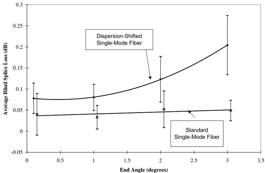
**Figure 1: The effect of end angle on splice loss**
