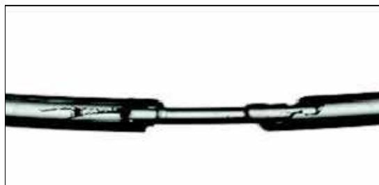
Figure 3 . Abrasive Damage of an Optical Fiber, Resulting in the Removal of the Fiber Coating and Exposure of the Cladding Surface
