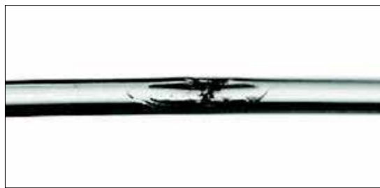
Figure 2. Compressive Damage of an Optical Fiber, Resulting in Splitting of the Polymeric Coating
