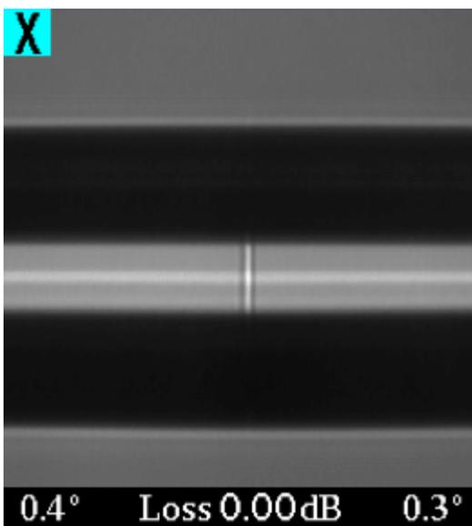
Figure 1. Homogeneous Splice
