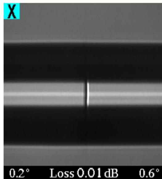
Figure 2. Heterogeneous Splice
