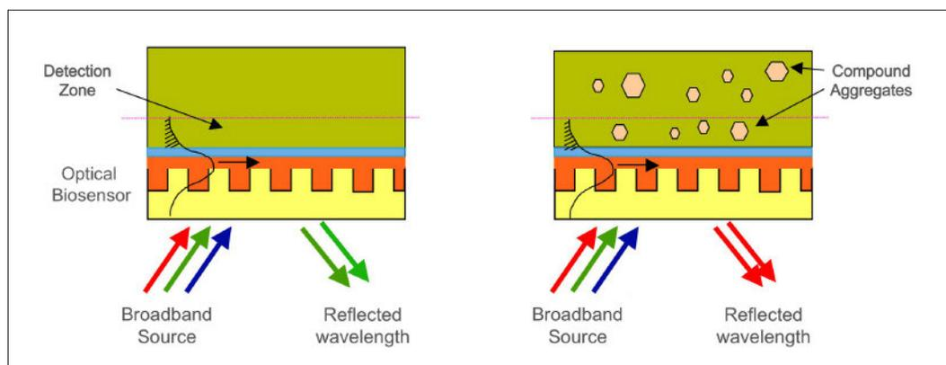
**Figure 1.** Epic Technology can detect compound aggregation using a simple add and read assay format. Uncoated Epic microplates containing integrated optical biosensors in each well are first soaked with assay buffer and a baseline measurement is taken. Compound is added in DMSO and aggregate formation at the surface of the biosensor is detected by measuring the wavelength shift of reflected resonant light.
