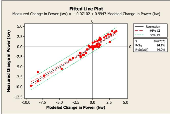
Chart 6 Regression Analysis Of Actual Changes In Horsepower Vs. Predicted Changes In Horsepower
