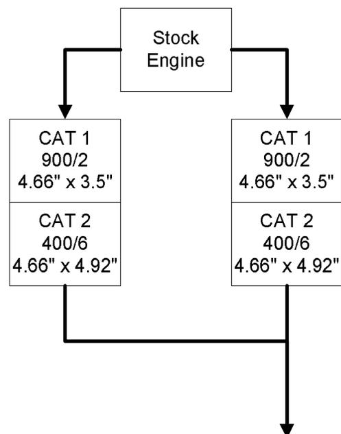
Figure 2 Stock Catalyst System Architecture
