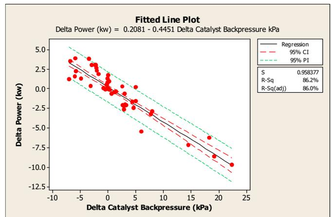
Chart 5 Effects Of Actual Measured Backpressure On Horsepower (Combined 75% And 100% Throttle)
