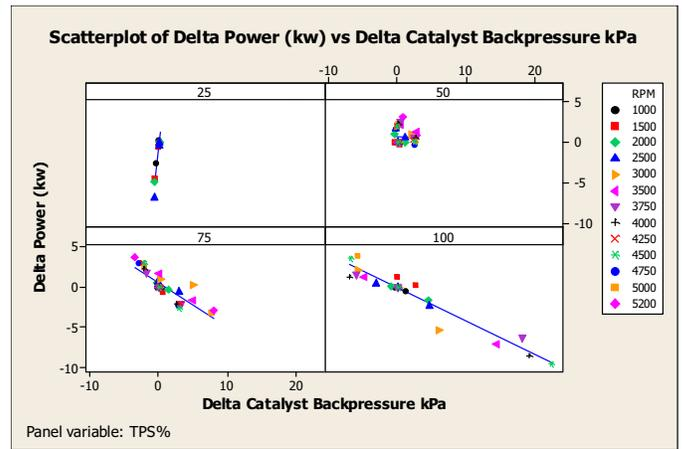
Chart 4 Effects Of Actual Measured Backpressure On Horsepower (All Throttle Conditions)
