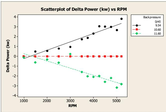
Chart 2 Horsepower at 75% Throttle Condition
