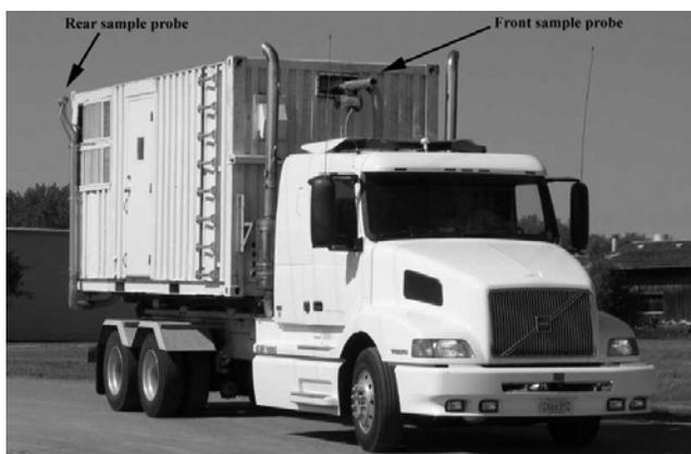
**Figure 4. Photograph of the Mobile Emissions Laboratory Used in The Present work.**
