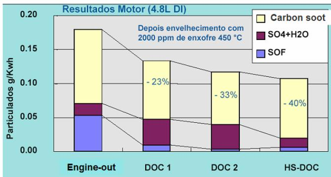
Figure 20. A new high sulfur DOC (HS-DOC) does not form sulfates in 2000 ppm sulfur fuel, despite high temperatures (76).
