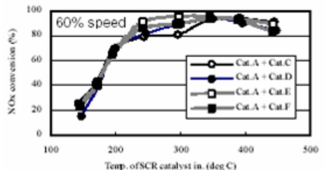
**Figure 5.** NO<sub>x</sub> removal efficiency curves for various SCR catalyst configurations (22). “Catalyst A” is an oxidation catalyst to promote the fast NO<sub>2</sub>/NO/NH<sub>3</sub> reaction. “Catalyst C” is vanadia-based, and the remaining catalysts are zeolite (25% smaller than the vanadia system).
