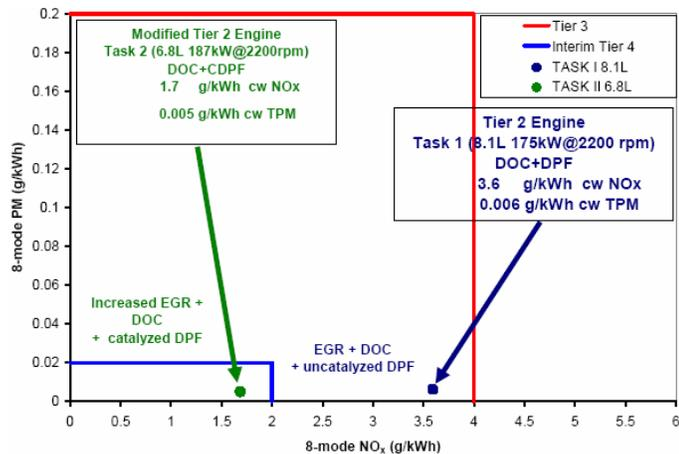
**Figure 23.** A interim Tier 4 (2011) non-road system, using high-pressure common rail fuel injection and cooled EGR to hit the NO<sub>x</sub> levels and a DPF to hit the PM levels. Fuel penalty is 3-5%. John Deere 6068H Tier 2 engine (83).
