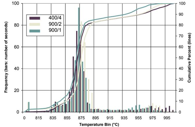
Figure 2: Histogram of bed temperatures 1 inch deep during aging
