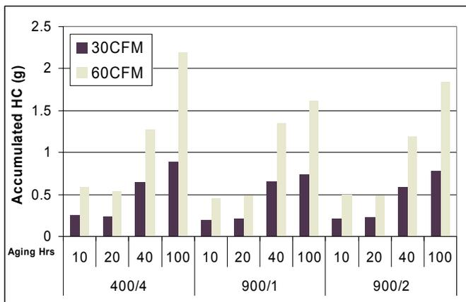
Figure 7: Comparison of accumulated hydrocarbons for both flow rates over steps in 100 hours of aging
