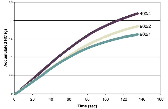
Figure 6: Accumulated Hydrocarbons - 100 hours of aging
