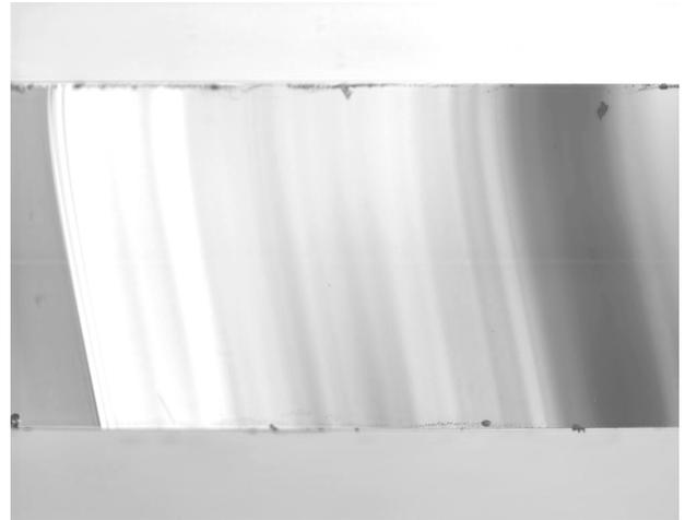
Fig. 9 Wallner lines on fracture surface Thermal stress is one stress that can generate this shape of Wallner lines. Crack run right to left.
