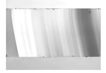
Fig. 9 Wallner lines on fracture surface Thermal stress is one stress that can generate this shape of Wallner lines. Crack run right to left.
