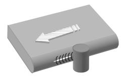
Fig. 12 Schematic illustration of the identified mechanism of origin creation on the case. Actually, glass sheet slides with direction of arrow mark with fixed pin, and relative rubbing direction by pin is opposite (left to right in this figure).
