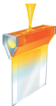
Figure 3. The Corning Fusion Process
