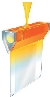
Figure 3. The Corning Fusion Process
