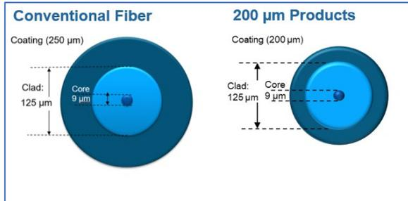
**Figure 1: Cross-sectional Comparison of Standard to 200  $\mu\text{m}$  Coated Diameter Fibres**
