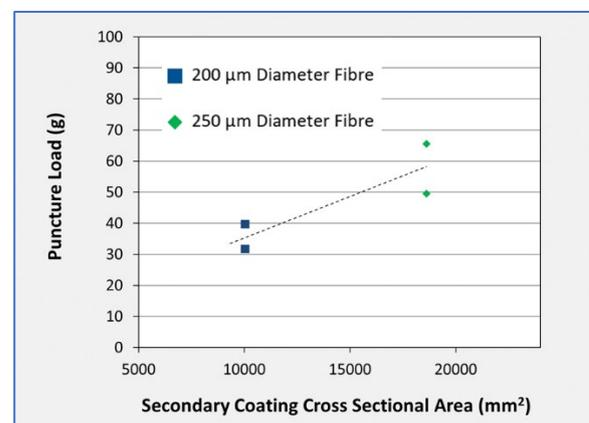
**Figure 4: Puncture Resistance Testing**
