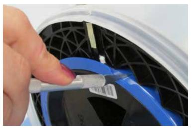
NOTE: In either method, it is important to collect and remove all stray fiber from the spool and surrounding area. This will help prevent fiber to fiber contact (whip) damage.
