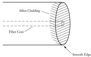
**Illustration of the Heating Effect on the Fiber End Due to a Burst Pre-fusion Cycle** Figure 5
