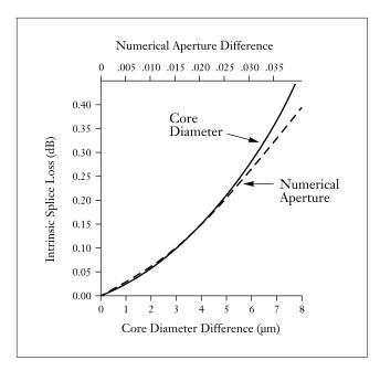
Note that the splice loss is directional with regard to these variables, i.e., loss occurs only when optical propagation is across a joint in which the receiving fiber has the smaller core diameter or NA. Splice loss values are additive, so if two multimode fibers that display mismatches in both core diameter and NA are joined, then their contribution to intrinsic loss is the sum of the two losses.
