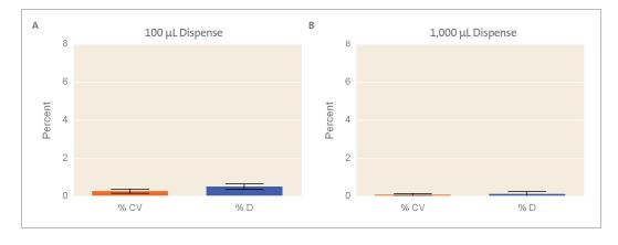
Figure 1. Analysis of HTF-1000-CBK-HTR-S tip with aqueous dispense. The precision (assessed by % CV) and accuracy (assessed by % D) of Axygen HTF-1000-CBK-HTR-S tips dispensing (A) 100 μL and (B) 1,000 μL volumes using the Hamilton Microlab STAR liquid handling workstation were determined using the Artel MVS® system. The % CV and % D were below 1.0 % for both 100 μL and 1,000 μL dispenses.
