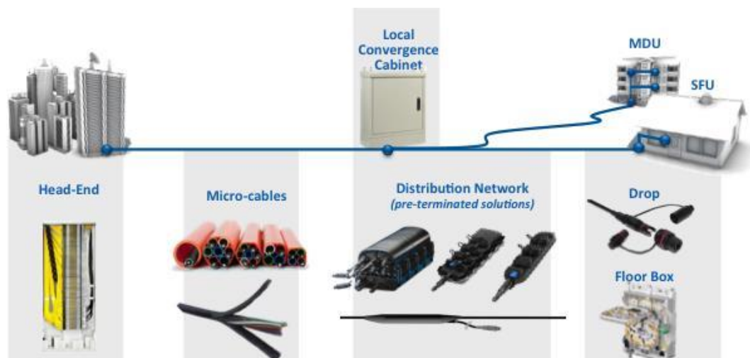
Solution components for the optimised network
