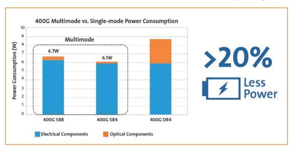
Figure 4. Multimode vs. Single-mode 400G Transceiver Power Consumption Comparison
