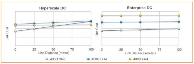
Figure 3: Link Cost Analysis for Hyperscale DC and Enterprise DC
