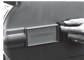
Unlock the red swivel lock as indicated on the sliding latch
