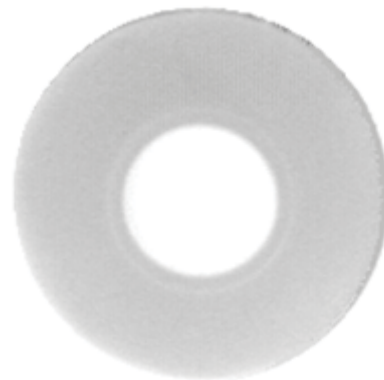
ClearCurve multimode fiber end-face (back-lit)
