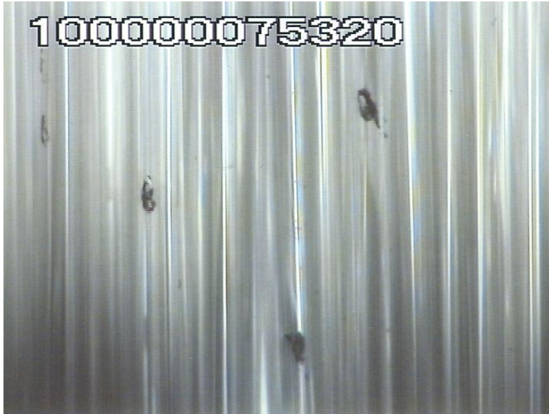
Illustration 1. Surface of a reel with surface blemishes generated by fiber end whip
