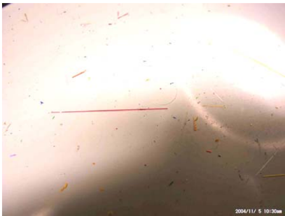
Illustration 6. A coloring surface contaminated by shards from previous break events
