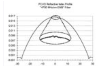
(See Appendix I) Fig 10: PCVD graded index profile.
