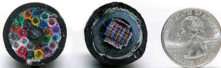
Loose Tube vs. Ribbon 288-Fiber Loose Tube (left) and 864-Fiber Ribbon (middle)
