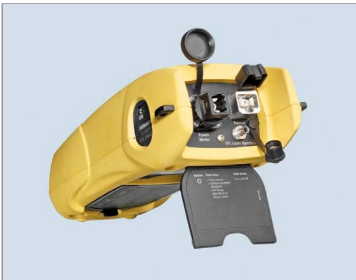
OTS 400 back view with SC connector adapters and VFL
