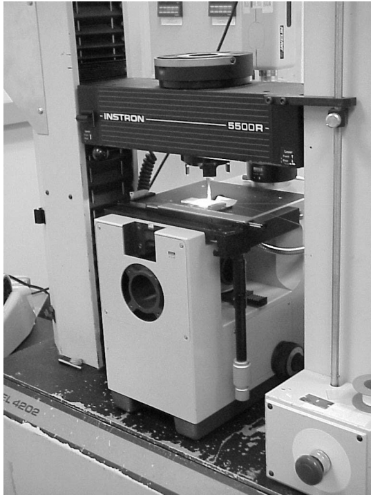
Figure 6. Testing machine outfitted with inverted microscope for indentation testing.
