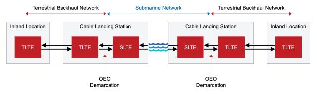
Figure 1: Distinct, yet interconnected, submarine networks and terrestrial networks.
