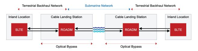
Figure 3: Simpler end-to-end network design via coherent optical transmission (GeoMesh Extreme).
