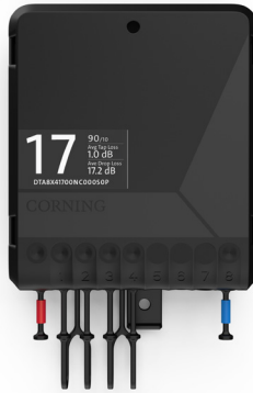
1x4 Optical Tap Terminal, 90/10 Power Split
