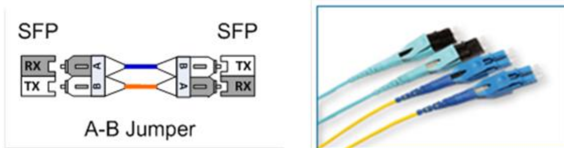
Figure 1: Duplex Fiber Optic Transmission
