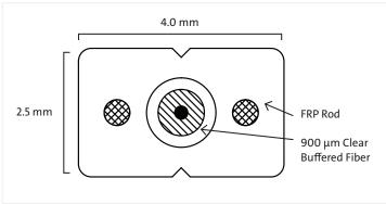
Isometric View of Clear Fiber Drop Cable
