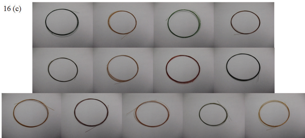
Figure 16. Images of optical fibers. From left to right, top row: blue, orange, green, brown; middle row: slate, white, red, black; bottom row: yellow, violet, rose, aqua, natural. (a) Fibers after 1800 hours (75 days) of 100°C aging in air. (b) Fibers after 336 hours (14 days) of 150°C aging in air. (c) Fibers after 24 hours of 200°C aging in air.
