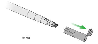
Step 3: Align the groove in the cleaner with the arrow on the connector and insert into the connector. Push on the cleaner until it clicks.
