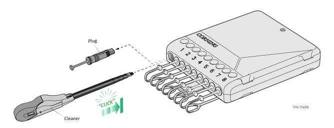
**Step 3:** Replace the dust plug, or follow the instructions in SRP-004-174-AEN for mating the connectors.
