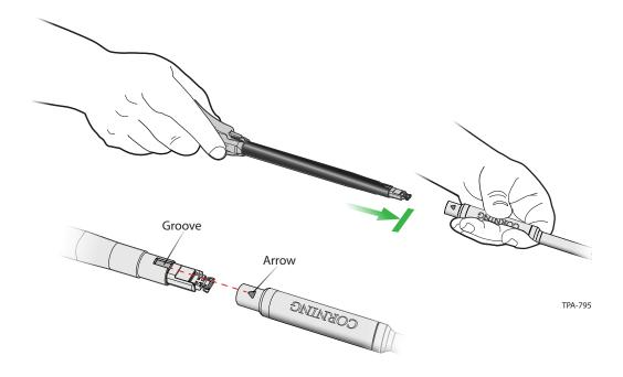
**Step 4:** Remove the cleaner and replace the connector dust plug.
