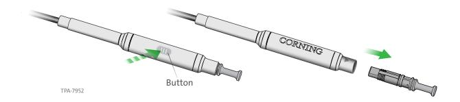
**Step 2:** Remove the adapter from the end of the cleaner.
