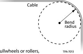
To find the minimum diameter requirment for bullwheels or rollers, simply double the minimum working bend radius
