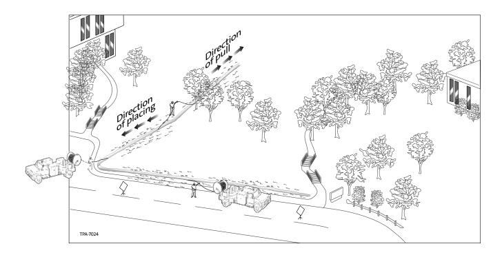
7.4 If the destination of the route is also inaccessible to vehicles, unreel and figure-eight the cable to gain access to the other end of the cable. Pull the cable into place with a stationary-reel method.
