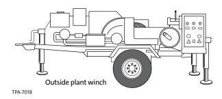
**NOTE:** Carefully select equipment that maintains bend radius. Not all outside plant equipment is well-suited for fiber optic cable installation.
