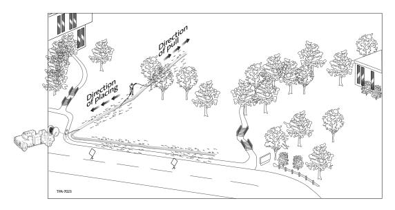
7.3 Following placement of this section, install the vehicle-accessible remainder of the cable route with the moving-reel method.
