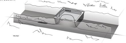
6.2 Various techniques are available to ease the installation of long lengths of fiber optic cable. The length of cable that can be pulled in one operation will vary with ground conditions, the equipment used, pulling technique selected, and the skill of the craftsmen. The preferred method is to hand pull, completing one span section at a time.
