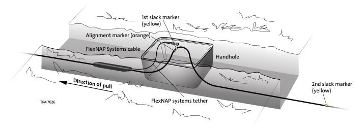
8.15 When a FlexNAP™ System tap point reaches its intended location, slow the pull speed. Each FlexNAP System tap point has an ORANGE alignment marker placed on the cable just after the FlexNAP System tap point.
