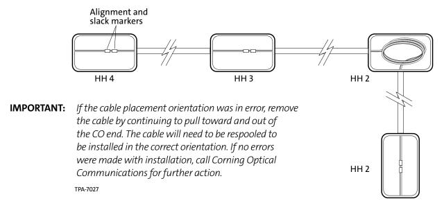
8.18 Also verify that the cable is placed in the correct direction. The tethers on the FlexNAP System cable are designed to point towards the "field" end of the cable, away from the CO/splice end.
