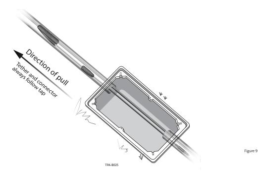
6.2 Various techniques are available to ease the installation of long lengths of fiber optic cable. The length of cable that can be pulled in one operation will vary with duct conditions, the equipment used, pulling technique selected, and the skill of the craftsmen. The preferred method is to hand pull completing one handhole/manhole at a time.
