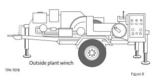
**NOTE:** Carefully select equipment that maintains bend radius. Not all outside plant equipment is well-suited for fiber optic cable installation.
