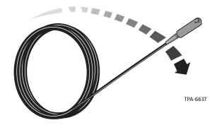
**WARNING:** Care must be taken to avoid cable damage during handling and placing. Fiber optic cable is sensitive to excessive pulling, bending, and crush forces. Any such damage may alter the cable's characteristics to the extent that the cable section may have to be replaced. To ensure all specifications are met, consult the specific cable specification sheet for the cable you are installing.
