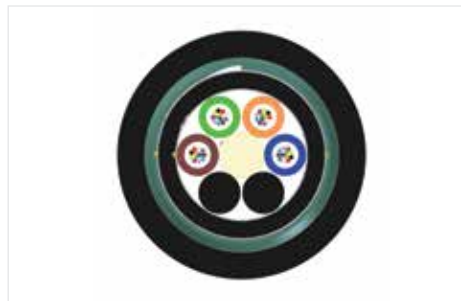
LSZH Armored Cable Cross Section
