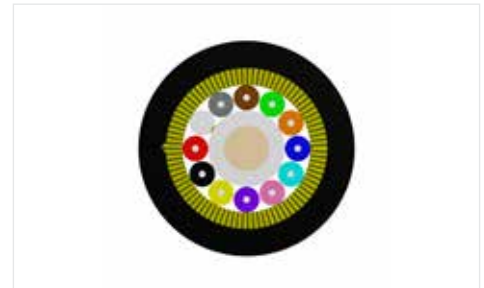
12 F FREEDM One Cable Cross Section
