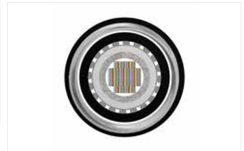
864 F LSZH Ribbon Gel-Free Interlocking Armor Cable Cross Section
