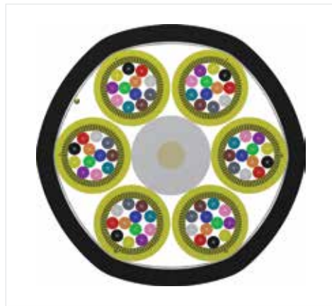
FREEDM One Cable Cross Section
