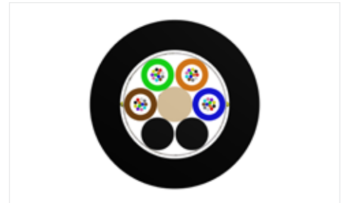
48 F FREEDM Loose Tube Cable Cross Section
