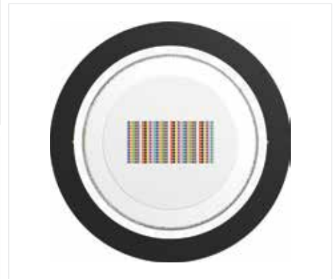
LSZH UltraRibbon Cable Cross Section
