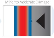
Surface flaws contained within compression layer do not propagate
