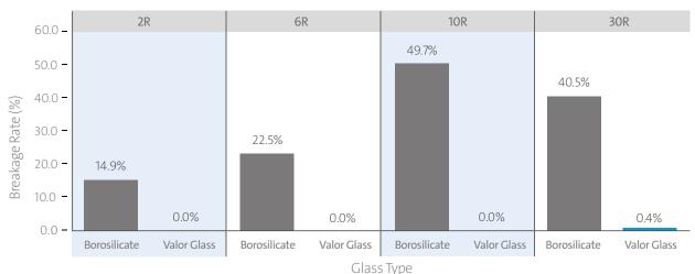
Freeze-thaw glass breakage rates using aggressive 15% mannitol with 50% fill volumes of 2R, 6R, 10R, 30R borosilicate vials compared to matching Valor containers. Study was conducted at -100°C to room temperature utilizing 1,000 vials/pedigree.
