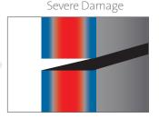
Deep checks propagate and complete the break separating into two or more pieces
