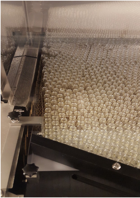
Figure 1 “En Masse” Movement of Glass on One of the First Trial Lines
