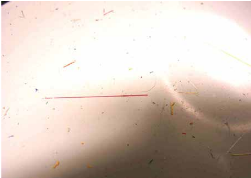
Figure 6. A coloring surface contaminated by shards from previous break events.
