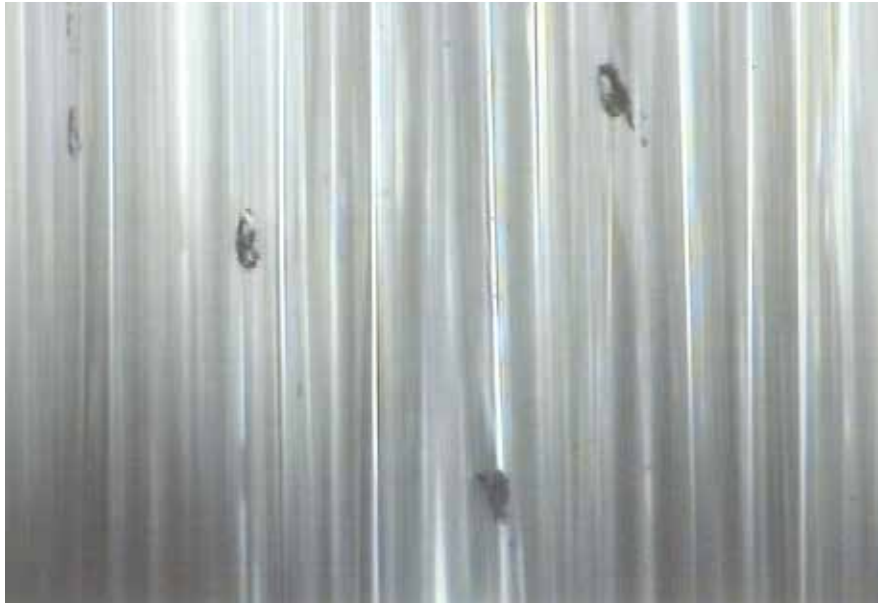
Figure 1. Surface layer of a spool under magnification with surface blemishes generated by fiber end whip.
