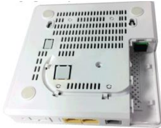
Model 1LAN-SDAN-8211 Rear View showing Optical connector SC/APC port, from the back side of the unit
